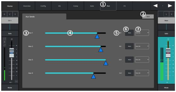
① AUX auxiliary transmit configuration interface.
